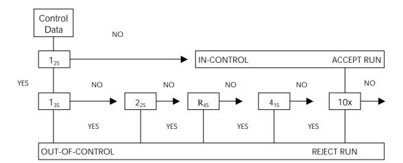
Figure 1. Quality Control Rule Diagram
